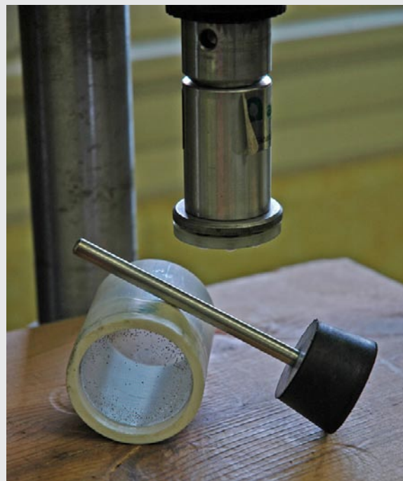
A drill press is transformed to aid in grinding cysts of Soybean Cyst Nematode. Photo Nancy Pataky
