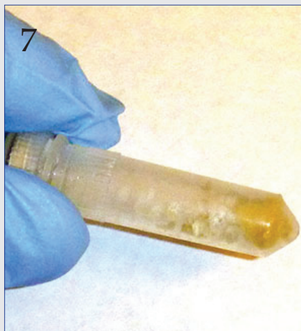
Fig. 5. Stick and tube are immersed in liquid nitrogen directly in the dewar. Fig. 6. Frozen tube is placed in Mini-BeadBeater-1 and ready for homogenization. Fig. 7. Microcentrifuge tube containing homogenized plant tissue.
