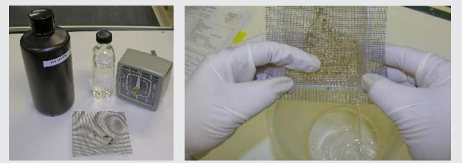
Figure 2 (left) Screen covering sample before surface sterilization. Figure 3 (right) Washing screens after use. Photos Meg Williamson
