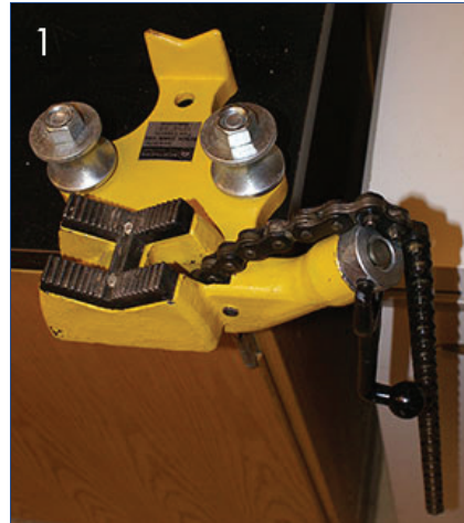
Fig 1. The bench chain vise is mounted on the right end of the counter. Mounting at the end of the counter is recommended since you turn a handle to tighten the chain. The composite material of lab benches is hard, so use a sharp drill bit and a drill with variable speed. We drilled slowly to prevent friction and damage to the counter.
