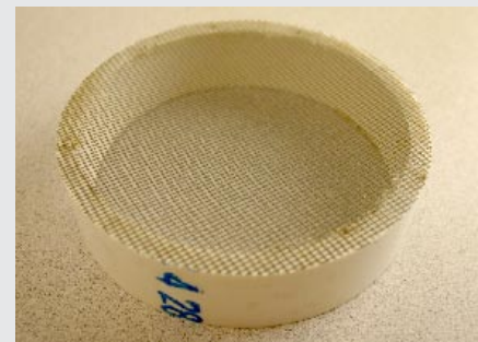
Figure 2. A cheap set of screens can be made by sawing off a 6 inch diameter PVC pipe into 1-2 inch segments, to which are glued circles of nylon window screening. (Photo Tom Creswell, NCSU)
