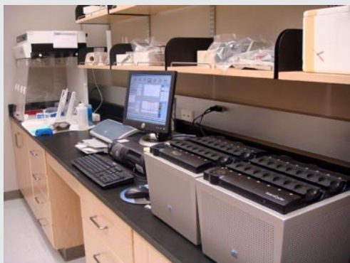
Figure 3. One side of the RT-PCR Room showing Cepheid RT-PCR System and Captair Bio by Erlab hood for DNA work.
